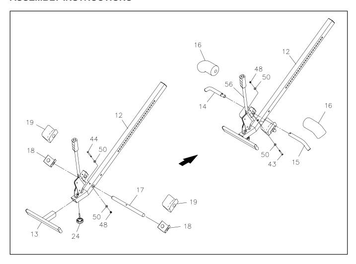
STEP 4: Attach the FOOTREST(13) onto the HEIGHT ADJUSTMENT BEAM(12) with the ADJUSTMENT KNOB(24).
